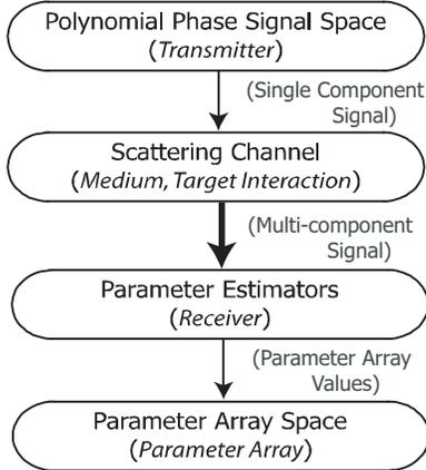
Fig. 6. Information Flow for Parameter Estimation
