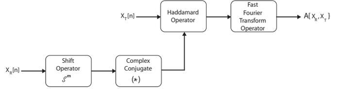
Fig. 7. Cross-Ambiguity Function Block Diagram
